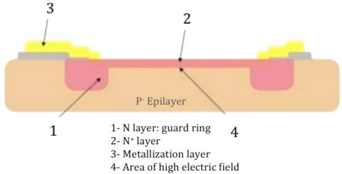
**Figure 1:** Geiger Photodiode structure based on N<sup>+</sup>/P junction and guard ring N layer.
