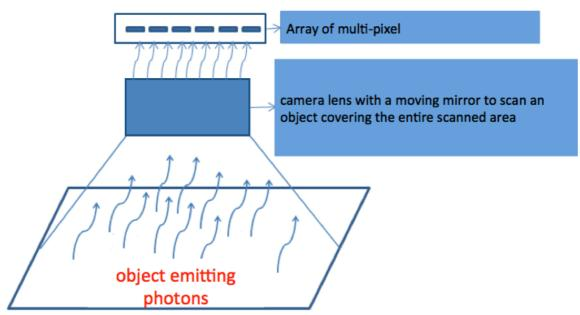
**Figure 3:** Illustration of detection system; photons are emitted by the scanned object and are collected by the lens which converge them to the detector (figure not to scale).
