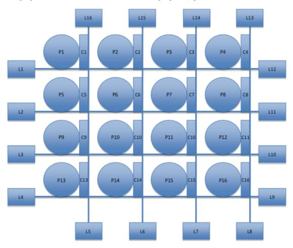
**Figure 2**: Illustration of an imaging system in CMOS 0.35μm Opto. An example of 4x4 photodiodes matrix, each photodiode has its read-out circuit.
