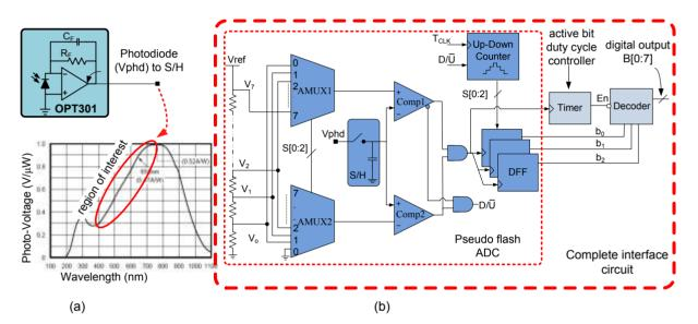
Figure 3. Proposed color sensor system (a) OPT301 photodiode and its gain adjustable photovoltage response. (b) Interface circuit of the color sensor.
