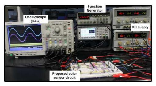
Figure 5. Experimental setup to test the proposed color sensor
