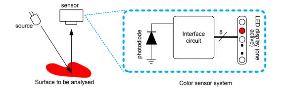
Figure 1. Surface color detection principle based on reflectance.
