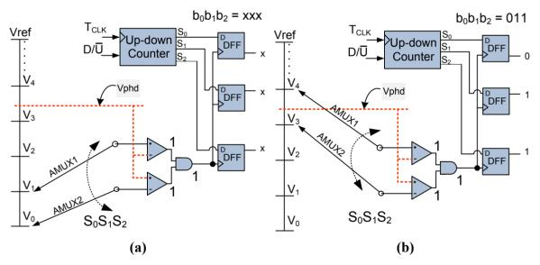
Figure 4. Conceptual diagram illustrating operation of the embedded ADC. (a) The AMUX's switch through the ladder voltage until both comparators fire, during this time the output is not updated from previous detection. (b) Both comparators fire indicating conversion process is completed.
